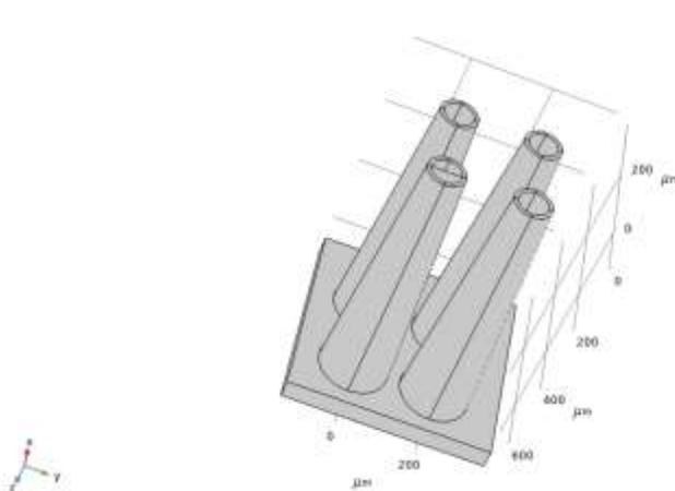
Fig. (1) Geometry of coated microneedles
