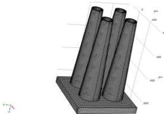
Fig. (2) Meshing of Microneedle
