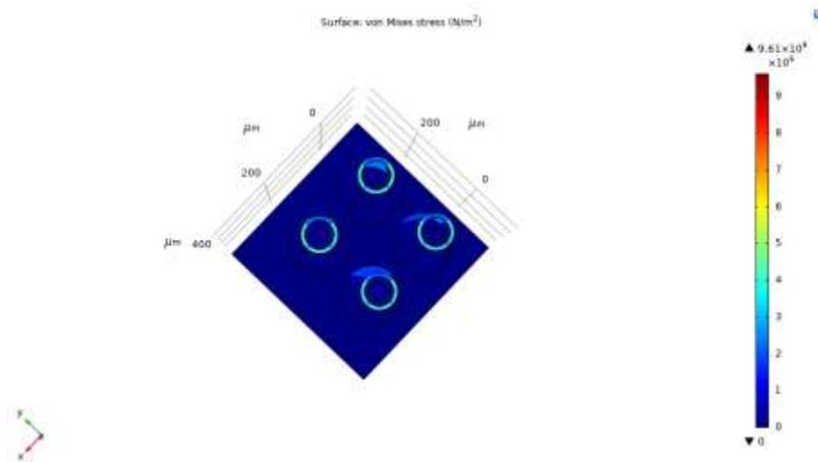
Fig. (3) Stress at Microneedle-Coating Interface
