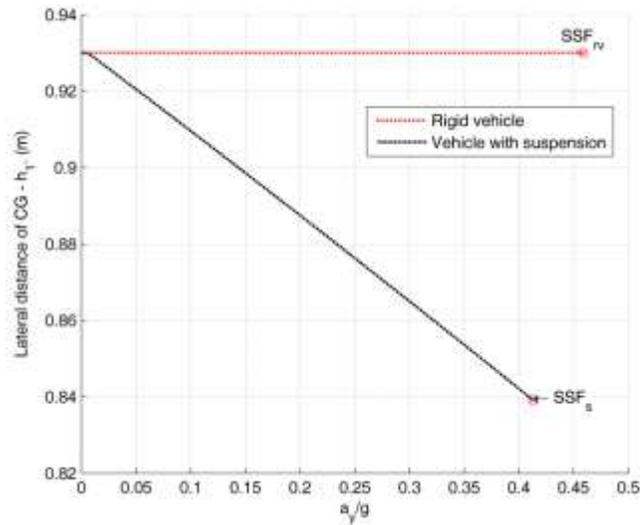
Figure 9. The instant lateral distance between the zero-reference frame and the center of gravity ( $h_1$ ).
