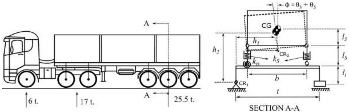
Figure 6. Parameters of heavy vehicle.
