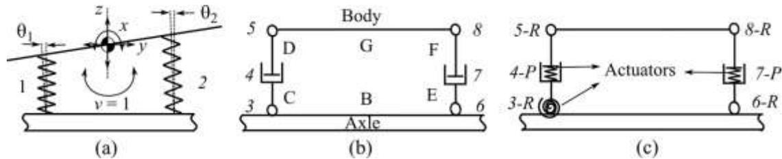
Figure 3. (a) Movement of the suspension system. (b) Kinematic chain of the suspension system. (c) Suspension system including actuators.
