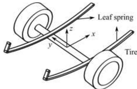
Figure 1. Solid axle with leaf spring [13].
