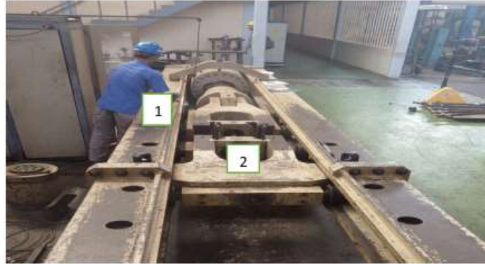
Figure 6. Position of (1) LVDT (2) anchor bolt
