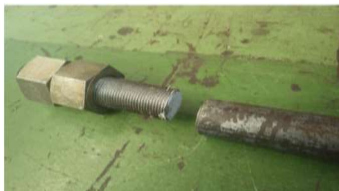
Figure 12. Test Result of Anchor Bolt
