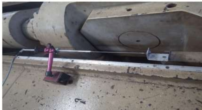
Figure 5. Position of LVDT placement on RH-Z machine
