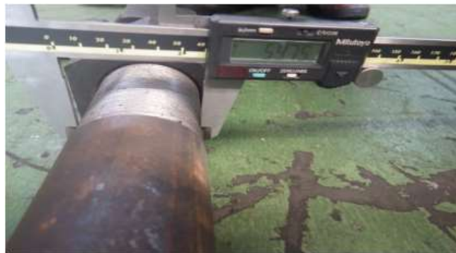
Figure 4. Inner diameter/threaded measurements of anchor bolt
