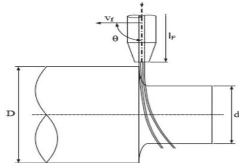
Fig 2 Schematic presentation of the AWJT process
