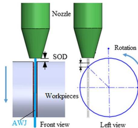
Fig 1. General principle of AWJT process
