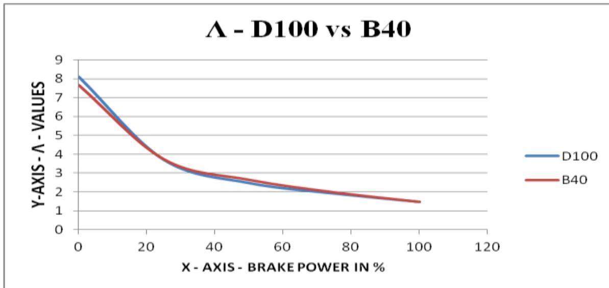
Figure 3: Lambda ( $\Lambda$ ) characteristic for D100 and B40
