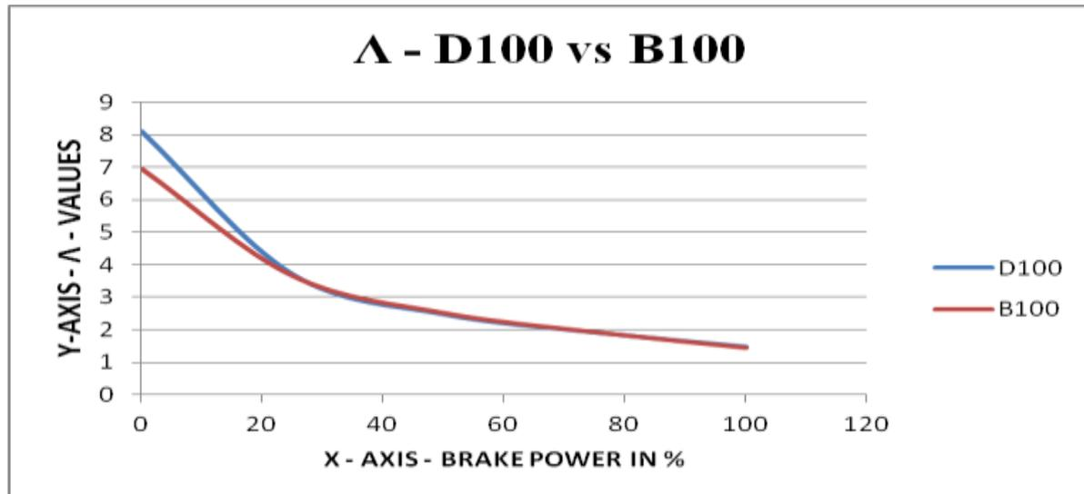
Figure 2: Lambda ( $\Lambda$ ) characteristic for D100 and B100
