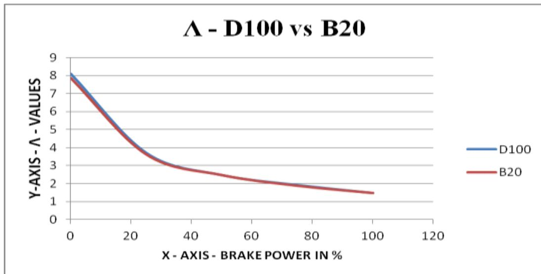
Figure 4: Lambda ( $\Lambda$ ) characteristic for D100 and B20
