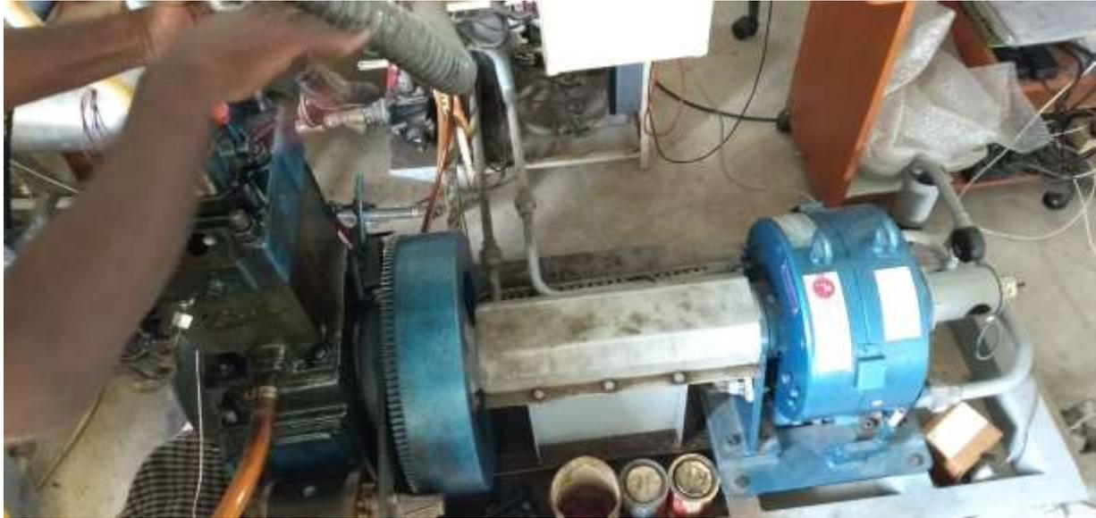
**Figure 1: Kirloskar Make – Single Cylinder Diesel Engine**
