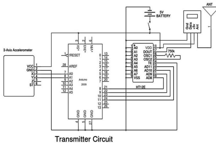
Fig 14. Transmitter circuit for the wheelchair system
