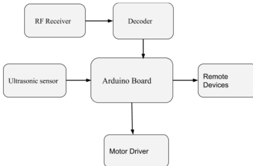
Fig 2. Block Diagram of Receiver
