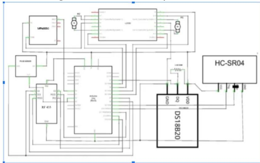
Fig 16. Overall circuit of the system
