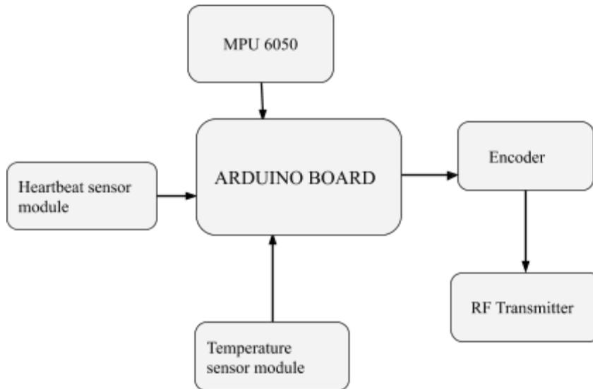
Fig 1. Block Diagram of Transmitter
