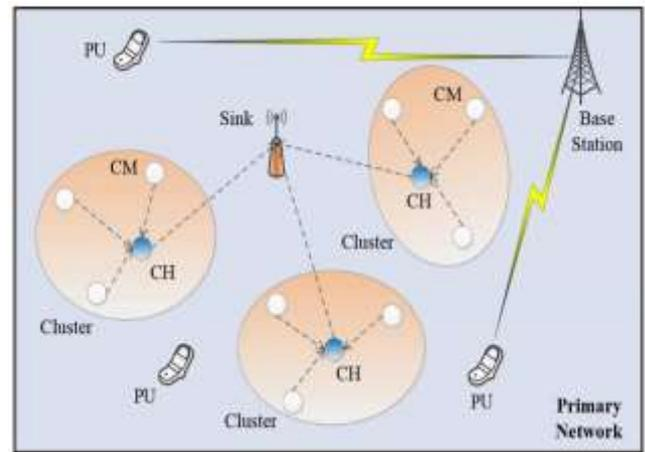
Figure 1: Architecture of cognitive radio sensor network
