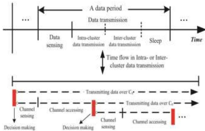
Figure 2: The time flow diagram of CRSN
