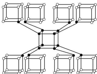
Figure 3: Crystal Structure Cubic Carbon (CC32)
