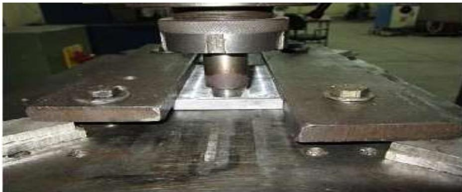
Figure 2 Friction Stir processing setup
