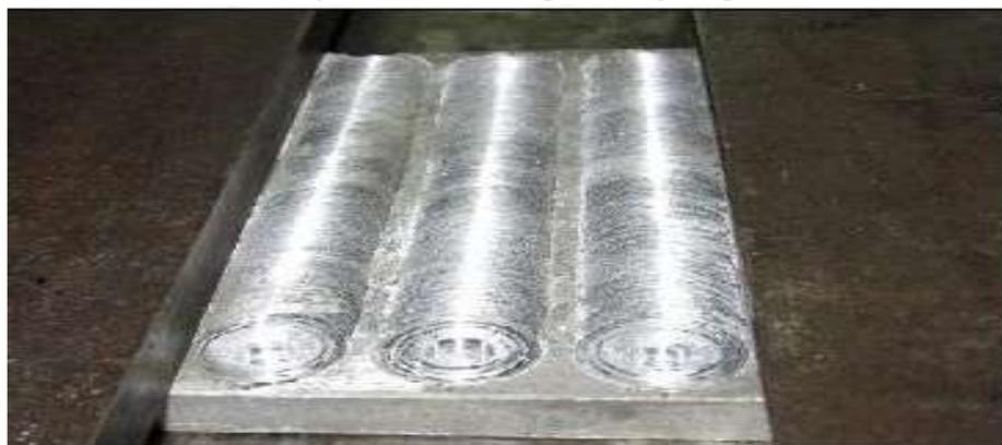
Figure 3 Friction Stir processing setup AZ91D alloy
