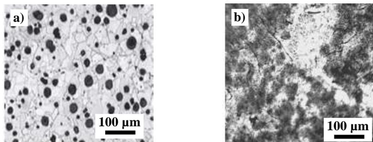
Figure 1. Microstructure comparison. a) Pearlite Nodular Foundry and b) Base material.
