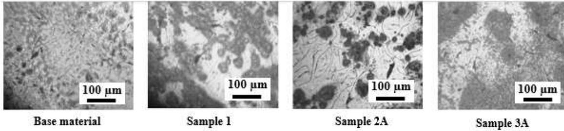
Figure 5. Metallographic samples with larger graphite size.
