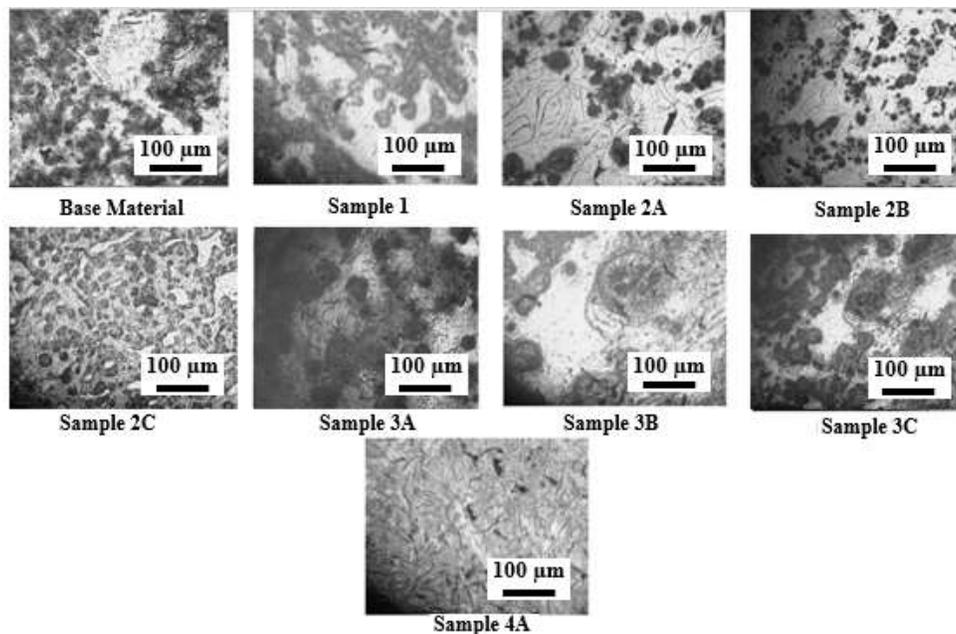
Figure 3. Metallography of the different specimens.
