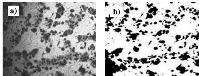
Figure 6. a) Annealed sample with a high presence of graphite nodules, and b) Modified nodular cast iron microstructure in ImageJ.
