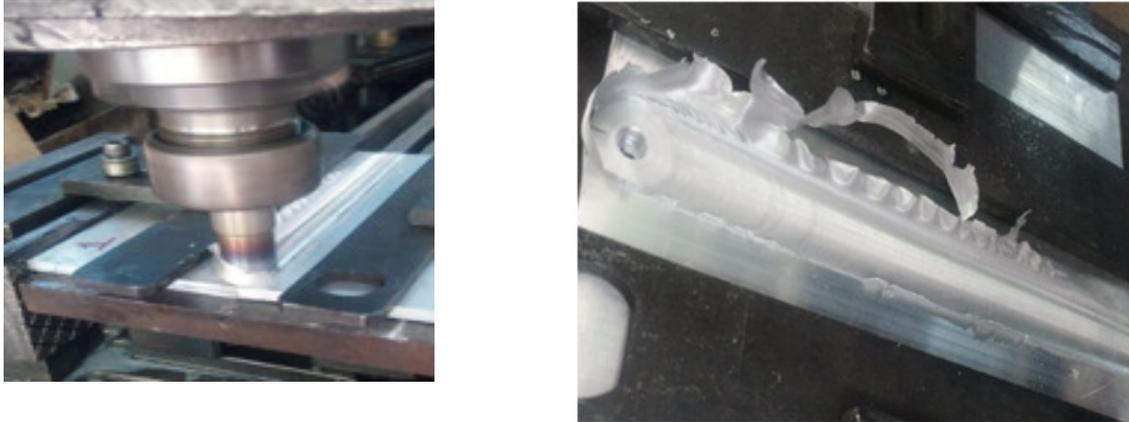
Figure 3: Friction Stir Welding of AA6061
