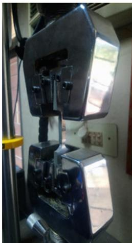
Figure 5: Tensile Testing on Nano UTM
