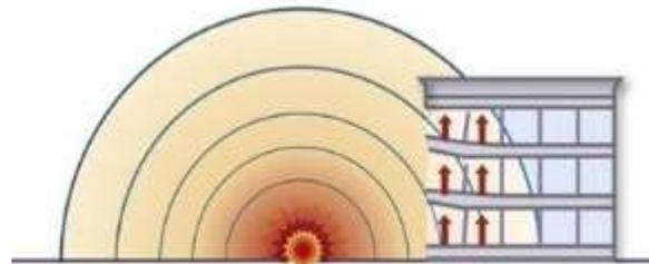
Figure 2. Blast wave with Moderate Damage Level
