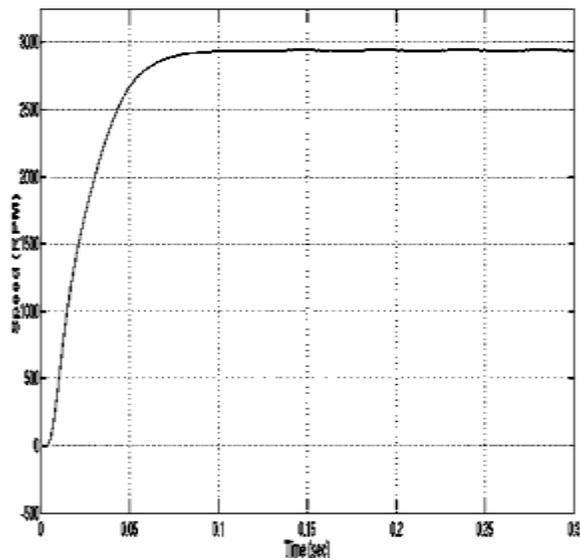
Fig.22.speed of the induction machine at 18 m/sec
