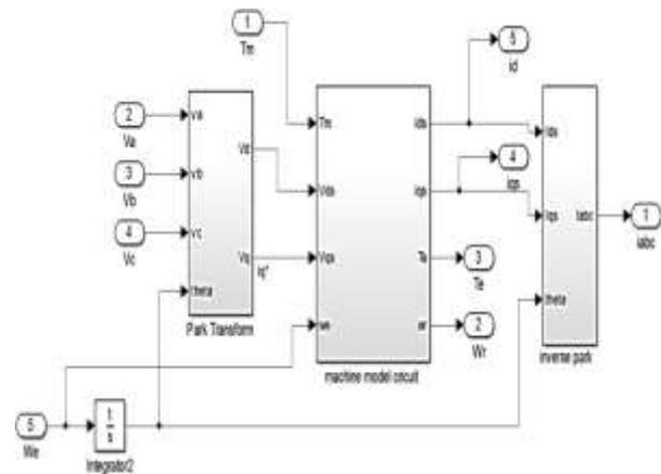
Fig.4.Simulation model of proposed induction machine
