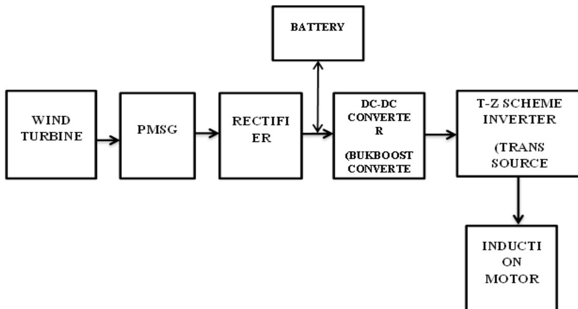
Fig.1.Block diagram representation of Proposed System
