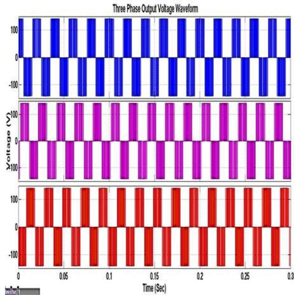
Fig.14.Three phase Output Voltage Waveform of Inverter
