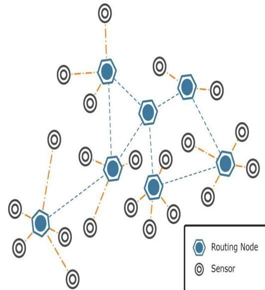
Figure 1: Representation of Wireless Sensor Nodes and Routing Nodes
