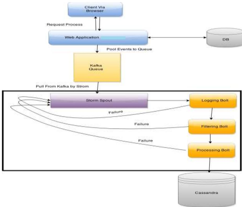
Figure 5.1.1 System Architecture Using Cassandra
