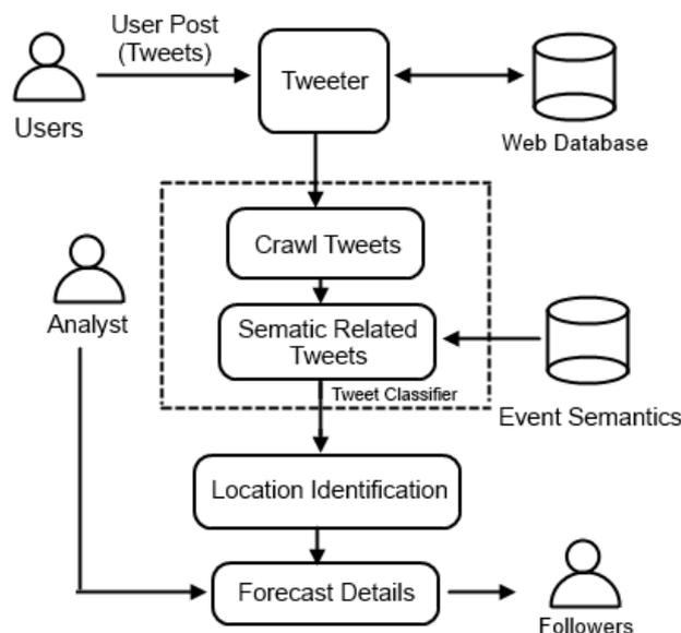
**Figure 5.1 System architecture**
