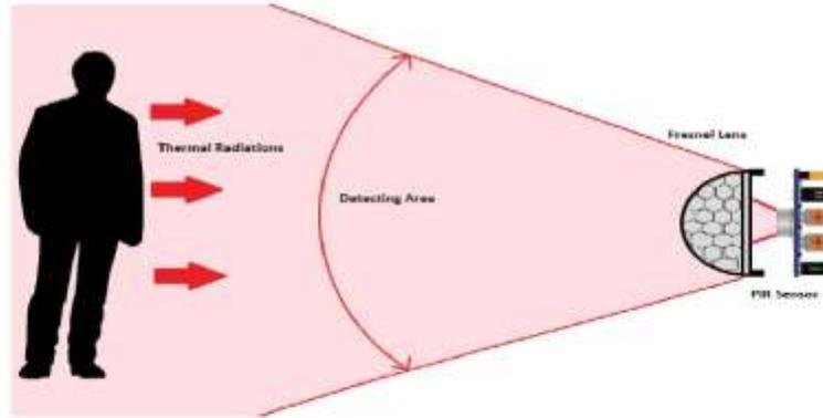
Fig. 3. Passive infrared sensor working
