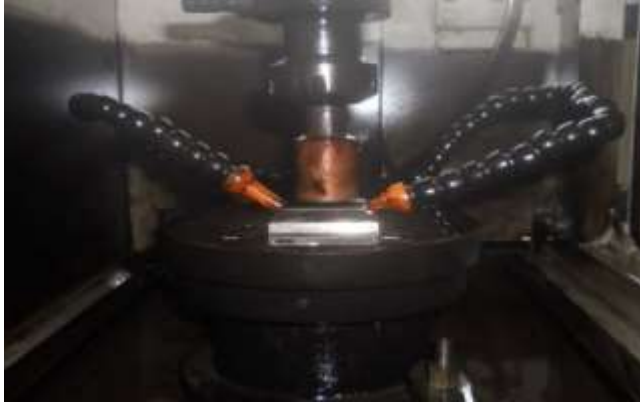
2: EDM apparatus Figure 3: Flushing position in EDM machine
