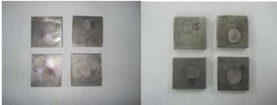
Figure 5: Machined surfaces of Aluminium with indent numbers
