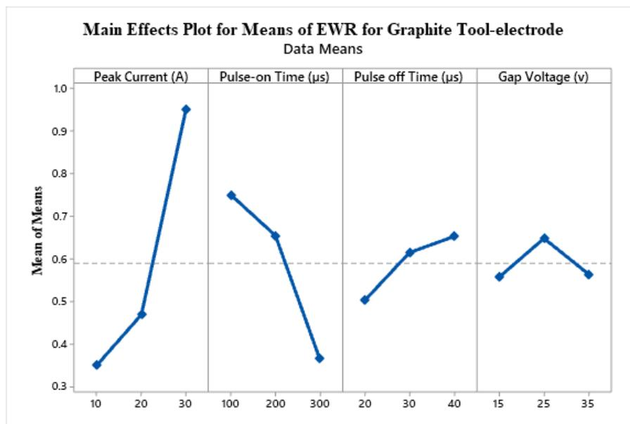
Figure 5. Main Effects Plot of EWR for Graphite Tool-electrode
