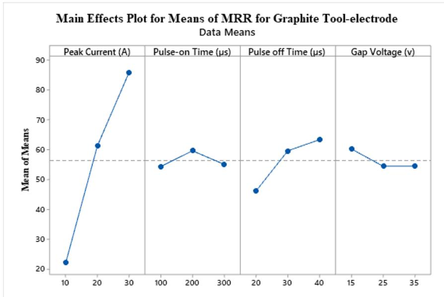
Figure 3. Main Effects Plot of MRR for Graphite Tool-electrode
