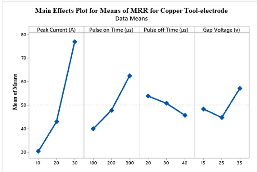
Figure 2. Main Effects Plot of MRR for Copper Tool-electrode
