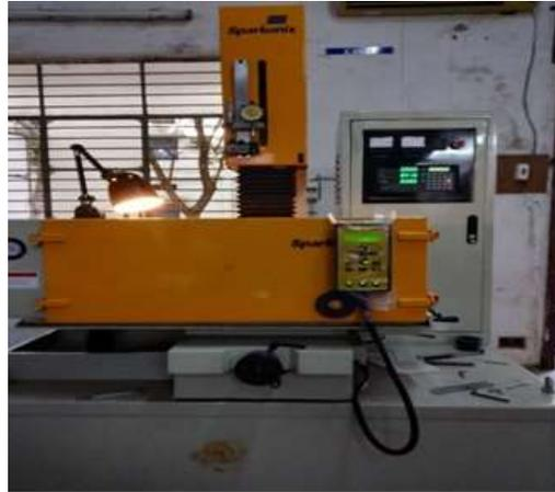
Figure 1. Die-Sinker EDM Machine (Make: Sparkonix S-35)
