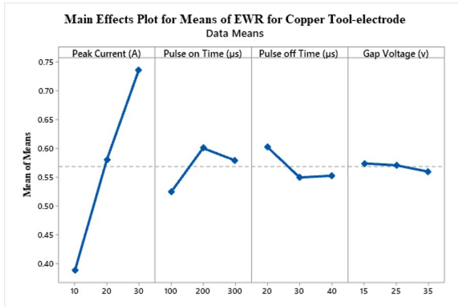
Figure 4. Main Effects Plot of EWR for Copper Tool-electrode
