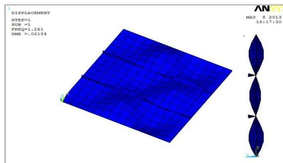
Fig 6. Buckling mode shape for P2R model
