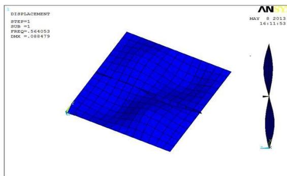
Fig 4. Buckling mode shape for P1R model
