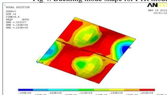
Fig 5. Stress contour diagram for P1R model
