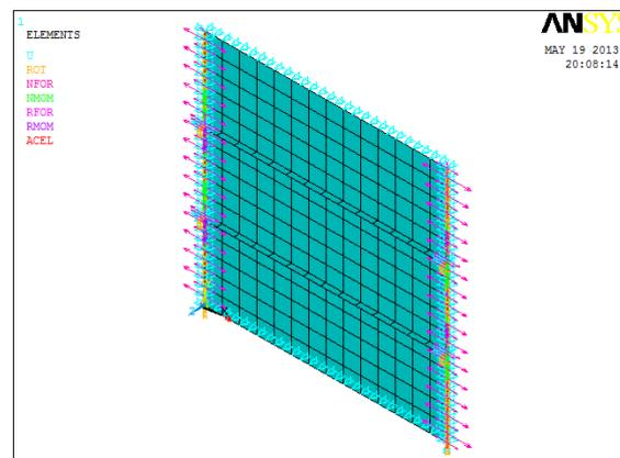
Fig 4. Boundary Condition for P2R Model
