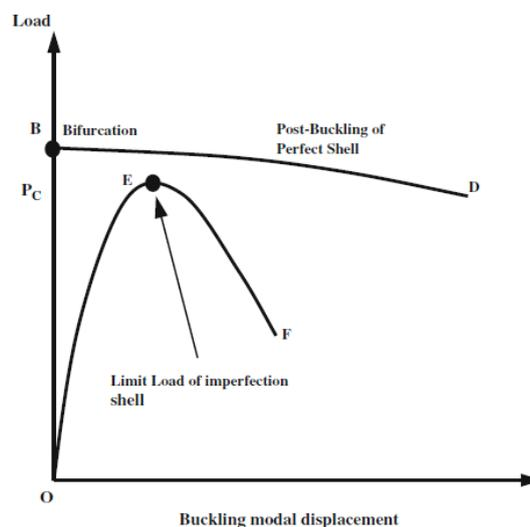
Fig. 2. FE analysis of eigen and non-linear buckling.
