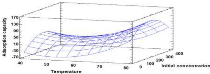
Figure 5. Response surface of Ni (II) ions adsorption under temperature and initial concentration variations
