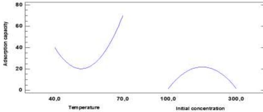
Figure 4. Influence of temperature and initial concentration of heavy metal ions on adsorption capacity
