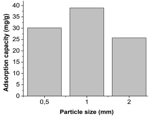
Figure 2. Effect of biomass particle size on adsorption performance
