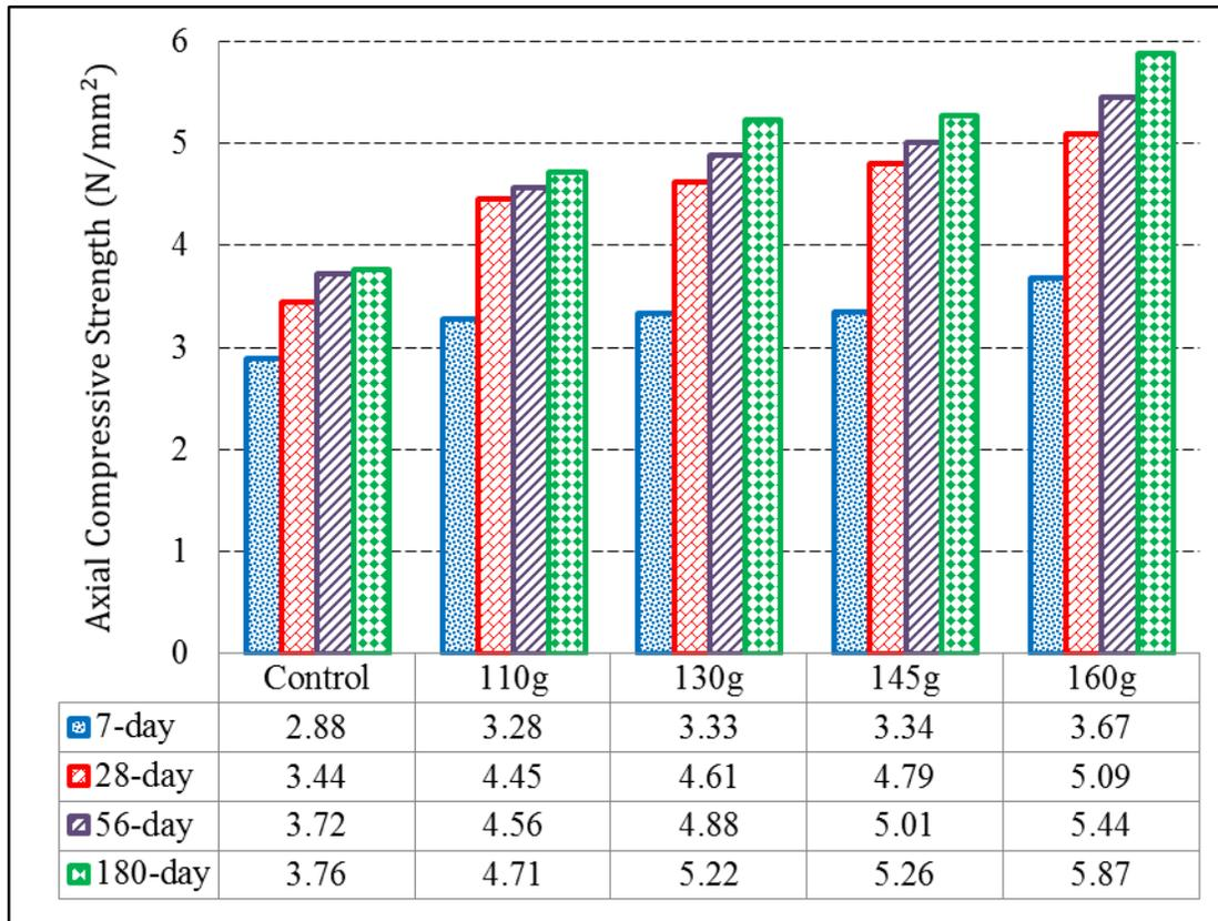
Figure 3 Axial compressive strength of LFC specimens confined with different weight of woven fibreglass mesh per area ( $\text{g/m}^2$ ).
