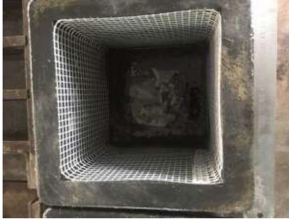
**Figure 1 Woven fibreglass mesh placed in mould.**
