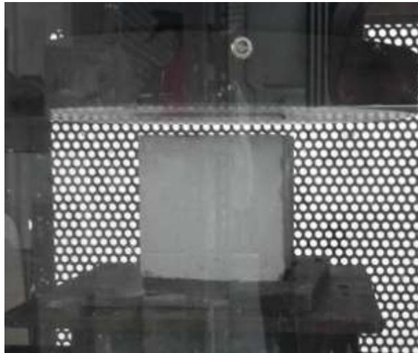
**Figure 2 Setup for compressive test using GOTECH GT-7001-BS300 Universal Testing Machine.**
