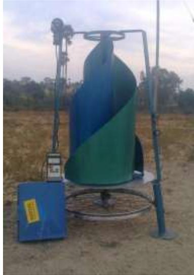
Utilized a supporting frame for the all involute spiral wind turbine parts are fitted with the supporting columns. The central mast is connected to a top side of the turbine soft bearing. Then central mast is also connected to the supporting arms. The supporting arms another end is connected to the turbine base plate. The turbine base plate are supported with three supporting columns.
