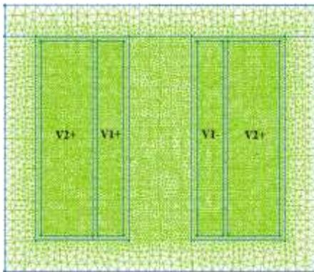
Fig. 4. 2D shell transformer meshed model
