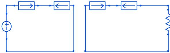
Fig. 3. Electrical equivalent circuit connections of windings
