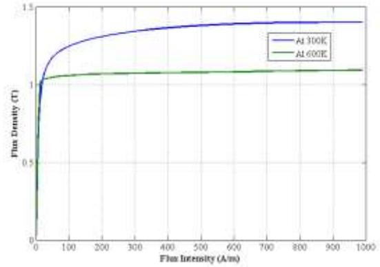
Fig. 5. B-H curve of the core at different temperatures
