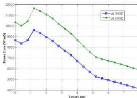
Fig. 8. Power loss in side limb in W/m<sup>3</sup>
