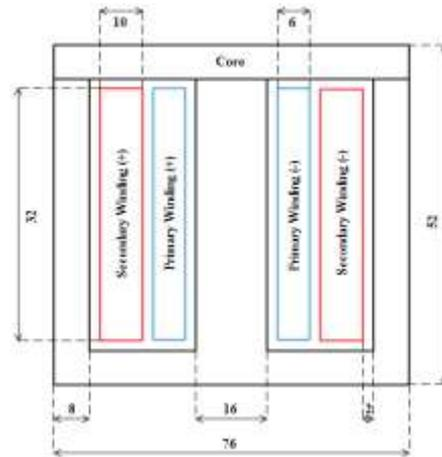
(b) Cut section view of 2D-Model
