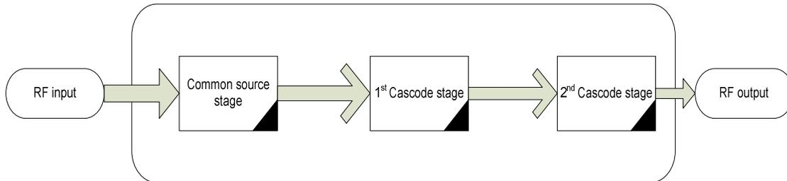
Fig 1. Block diagram of proposed Low noise amplifier
