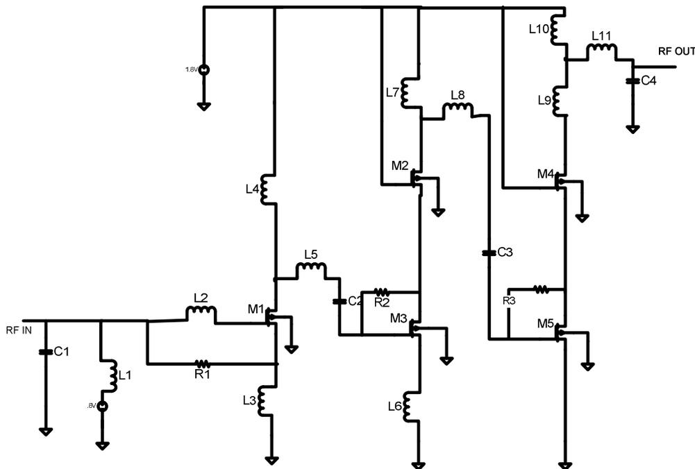
Fig.6 Proposed schematic of Low noise amplifier
