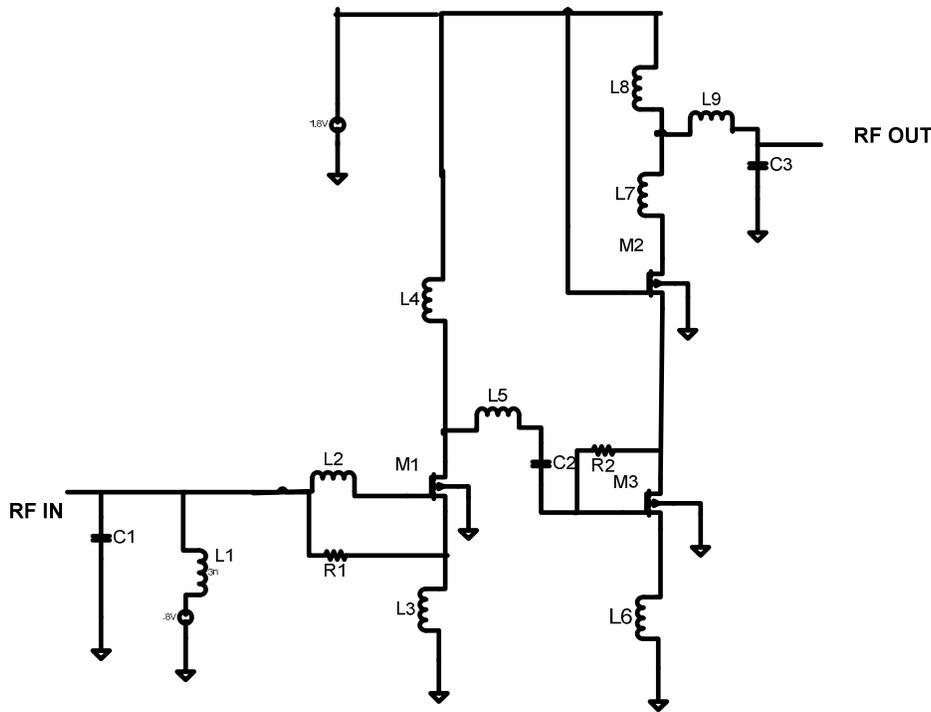
Fig.5 Conventional circuit of Low noise amplifier
