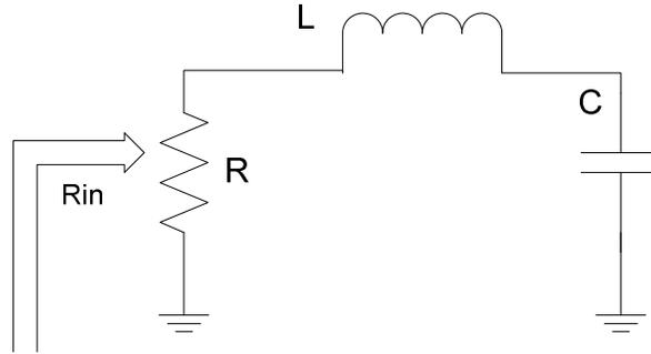
Fig.3 Input matching network of circuit
