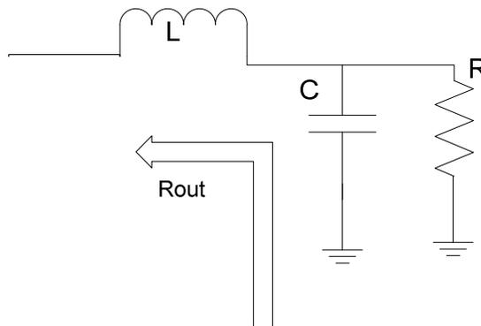
Fig.4 Output matching network of circuit
