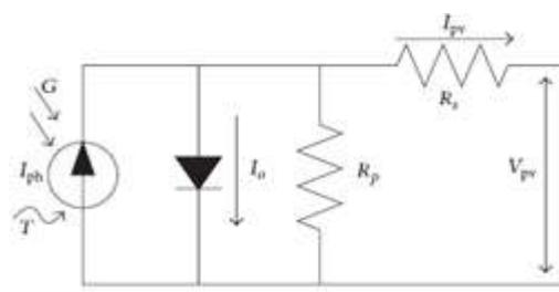
Fig 1 Equivalent Circuit of a PV Cell
