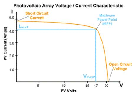
Fig 2 PV Cell Characteristics
