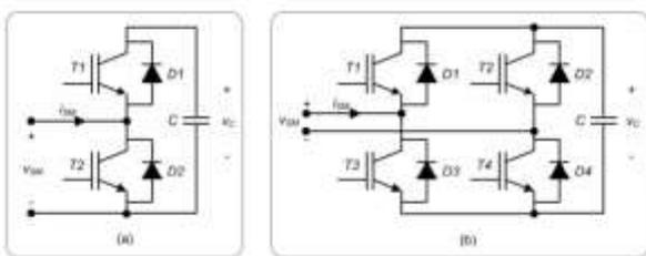
Fig 3. Switching module (SM) topologies: (a) half bridge; (b) full bridge
