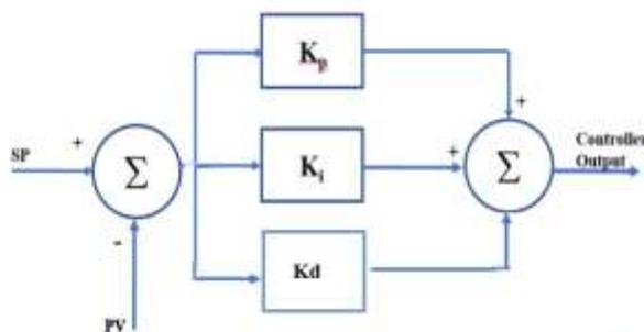
Fig 4. PID control block diagram
