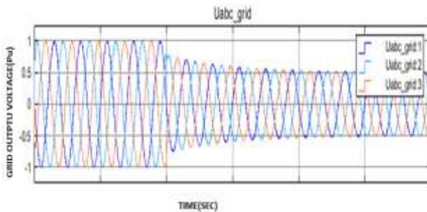
Fig 8. Grid output voltage with step response of 1-0.5 pu with step time of 0.1
