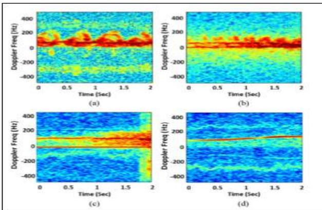
Figure 3. Spectrogram of moving targets (a) human (b) Buffalo (c) bicycle (d) car
