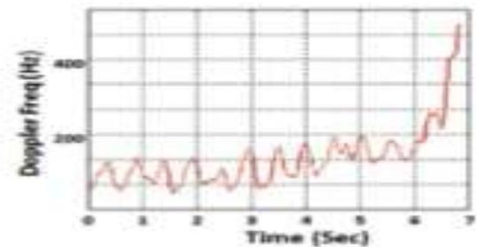
Figure 5 (b) detected envelope of the micro-doppler
