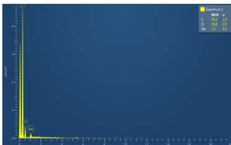
Figure 9: EDS images of (a) untreated fiber (b) treated fiber with NaOH
