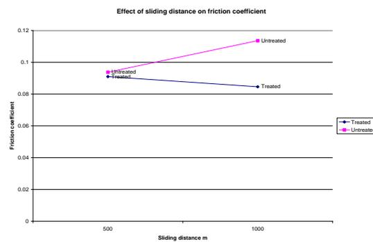
Figure 16. effect of sliding distance on friction co-efficient
