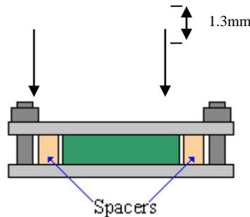
Figure 5. Compression set at 10% deformation of its length
