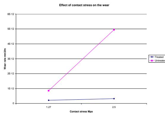
Figure 10. Effect of conduct stress
