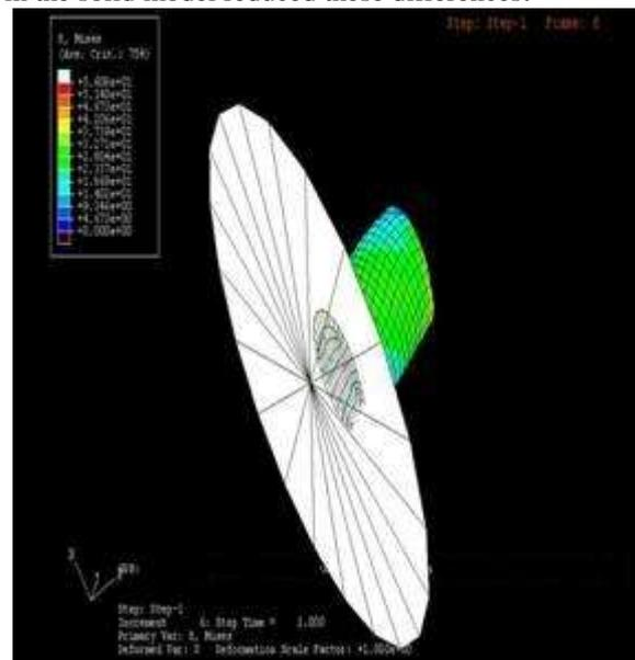
Figure 2. Vonmises stress when the load is maximum
