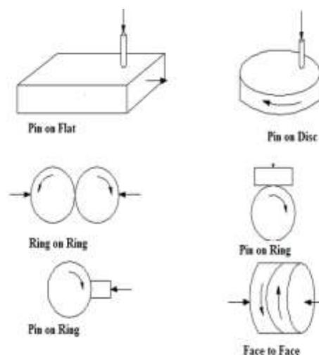
Figure 3. Geometries Employed in Sliding Wear Test.
