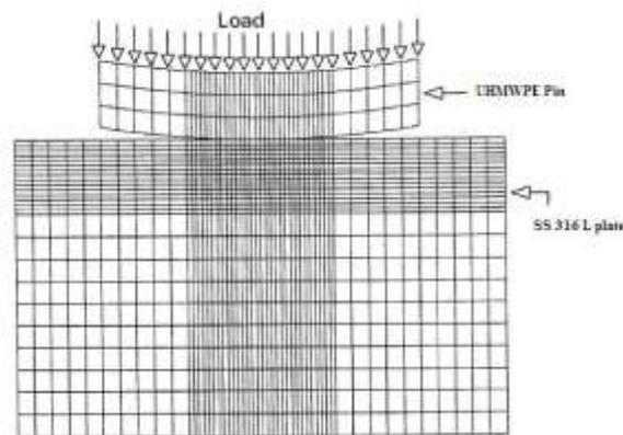
Figure1. FEA mesh model of contact pair
