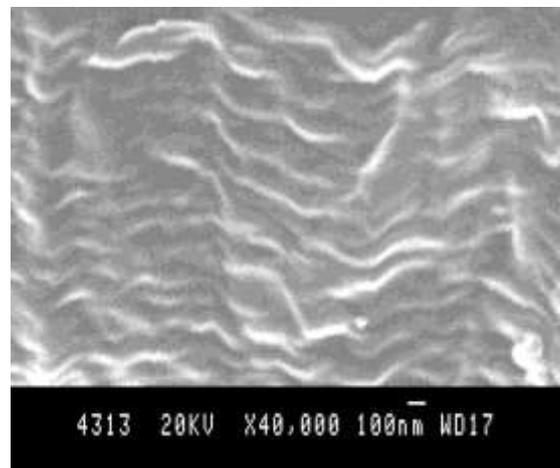
Figure 18. UHMWPE (Treated Sample)
