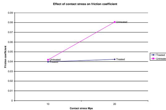
Figure 14. Effect of contact stress on friction co-efficient
