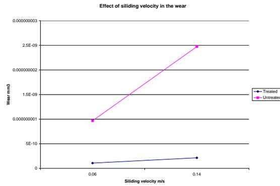
Figure 11. Effect of sliding velocity
