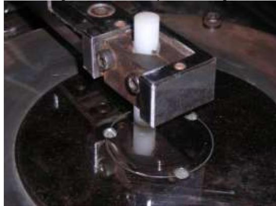
Figure 4 . Wear test rig-UHMWPE in pin holder and SS 316 L disc in the disk holder
