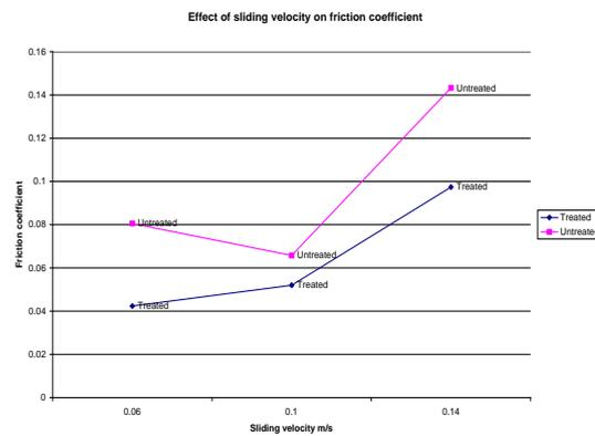
Figure 15. effect of sliding velocity on friction co-efficient
