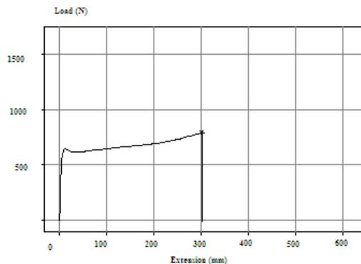
Figure 7. Tensile test graphs for Cryogenic Treated Material-1
