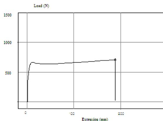
Figure 6. Tensile test graph for untreated UHMWPE material
