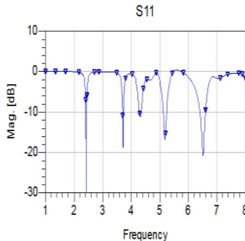
Figure. 4 Reflection Coefficient (S11) plot for proposed design
