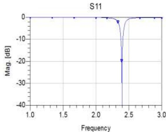
Figure. 2 Reflection Co-eff Vs Frequency for the basic antenna
