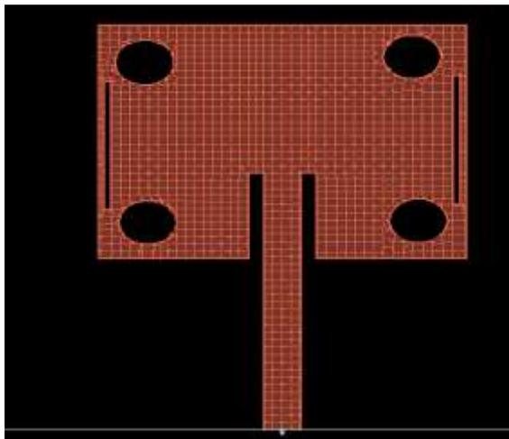
Figure. 3 Modified Patch with Circular slots and Vertical Slits
