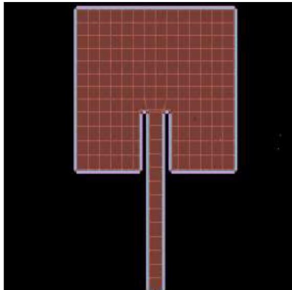
Figure. 1 Structural Top View of Patch
