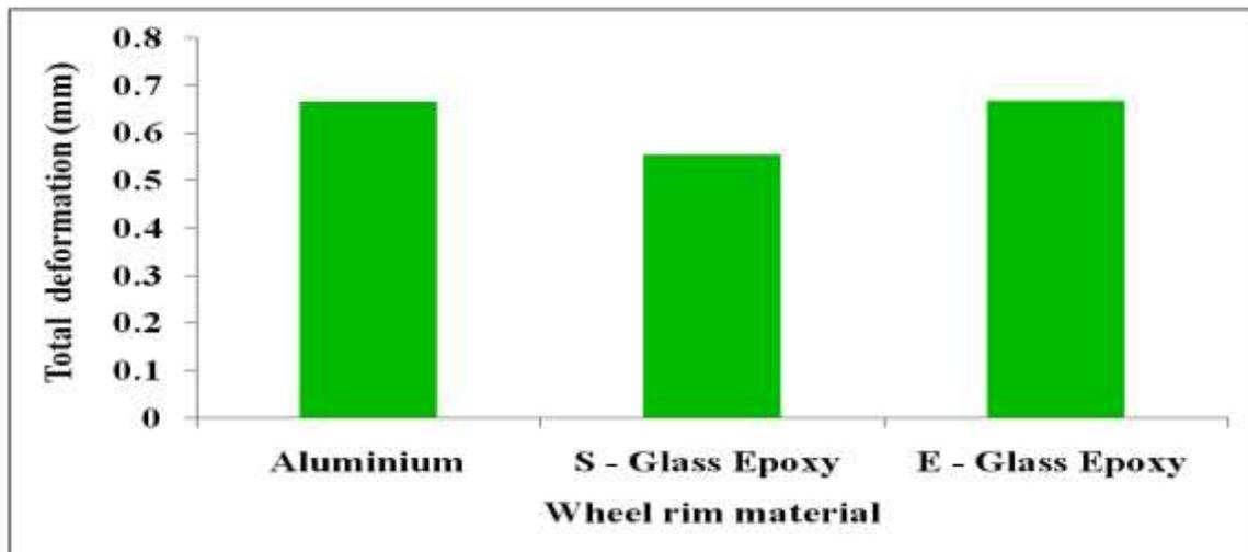
Figure 10 Maximum total deformation attained by the wheel rim for Aluminium Alloy 6061, S-Glass Epoxy and E-Glass Epoxy material
