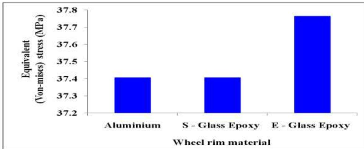
Figure 16 Distribution of equivalent Von-mises stress in Aluminium Alloy 6061, S-Glass Epoxy and E-Glass Epoxy wheel rim
