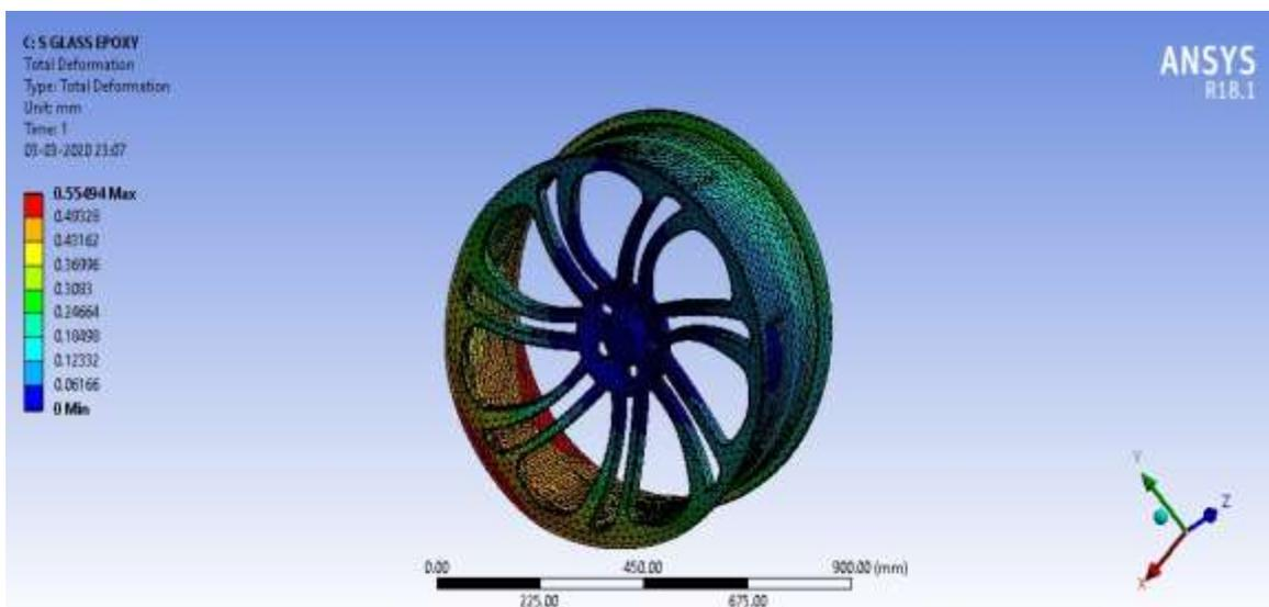
Figure 6 Total deformation under the applied load for S Glass Epoxy Wheel rim
