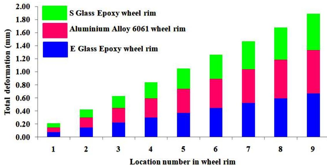
Figure 9 Minimum to maximum deformation exposed by S-Glass Epoxy, Aluminium Alloy 6061 and E-Glass Epoxy wheel rim
