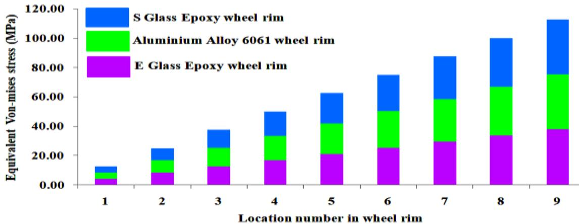
Figure 15 Minimum to maximum equivalent Von-mises stress exposed by S-Glass Epoxy, Aluminium Alloy 6061 and E-Glass Epoxy wheel rim
