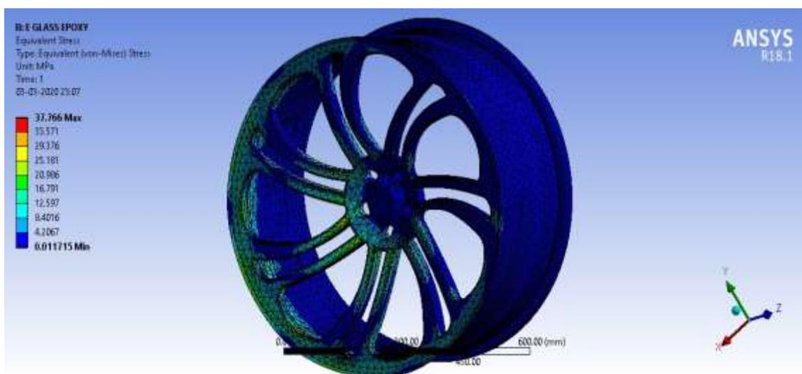
Figure 13 Equivalent Von-mises stress distribution in E-Glass Epoxy wheel rim
