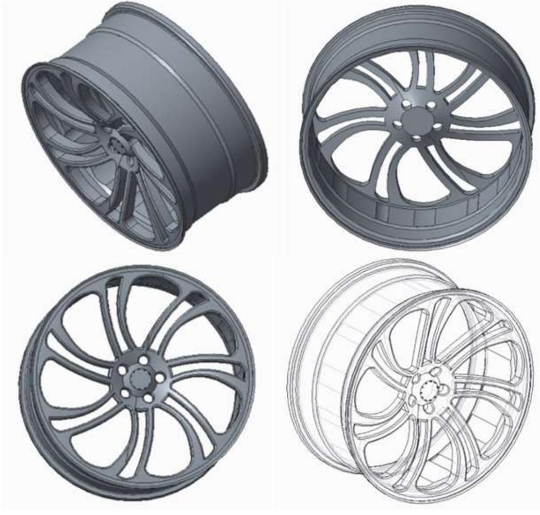
Figure 1 Comprehensive three-dimensional and wire frame model of an unmodified automobile wheel rim
