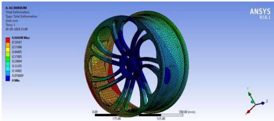
Figure 5 Total deformation attained by the Aluminum Alloy 6061 wheel rim
