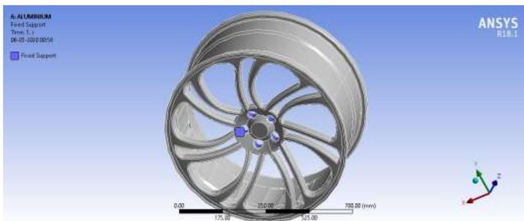
Figure 3 Wheel rim with applied boundary conditions for fixed support
