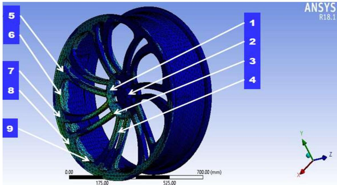
Figure 14 Minimum to maximum equivalent Von-mises stress attained by the wheel rim with corresponding location number
