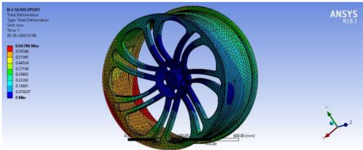
Figure 7 Total deformation of E-Glass Epoxy wheel rim under the applied loading condition
