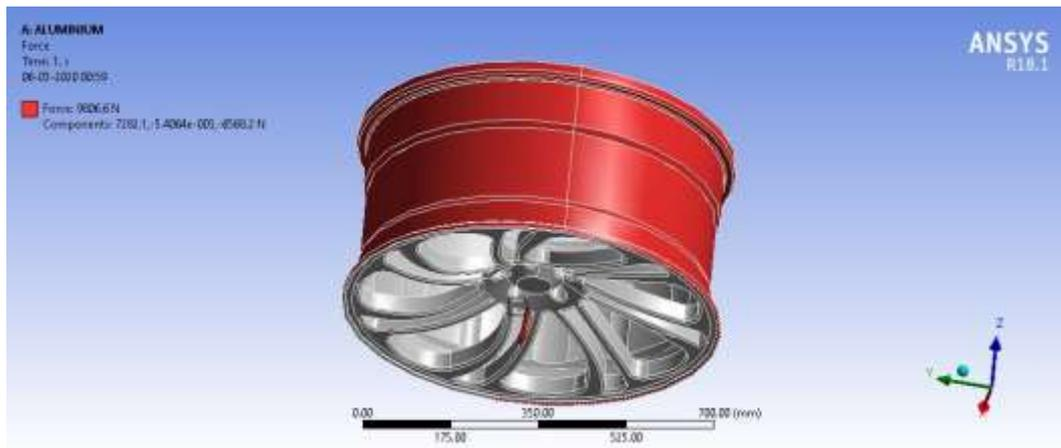
Figure 4 Wheel rim with force applied boundary conditions
