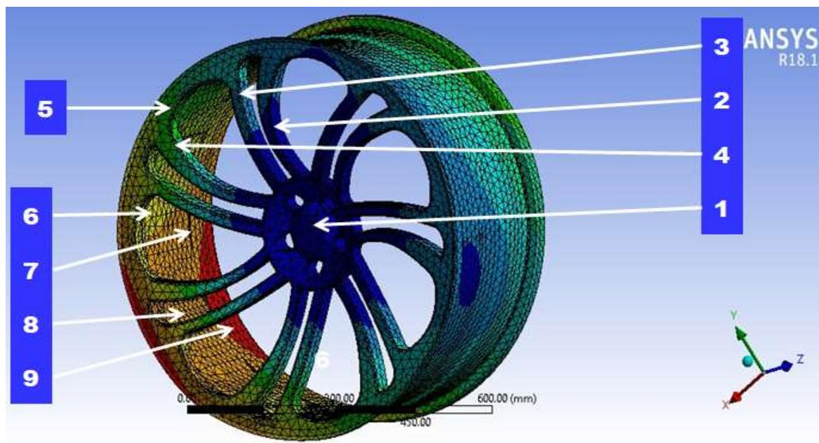
Figure 8 Representation of location wise deformation accomplished by the wheel rim from minimum level to maximum level
