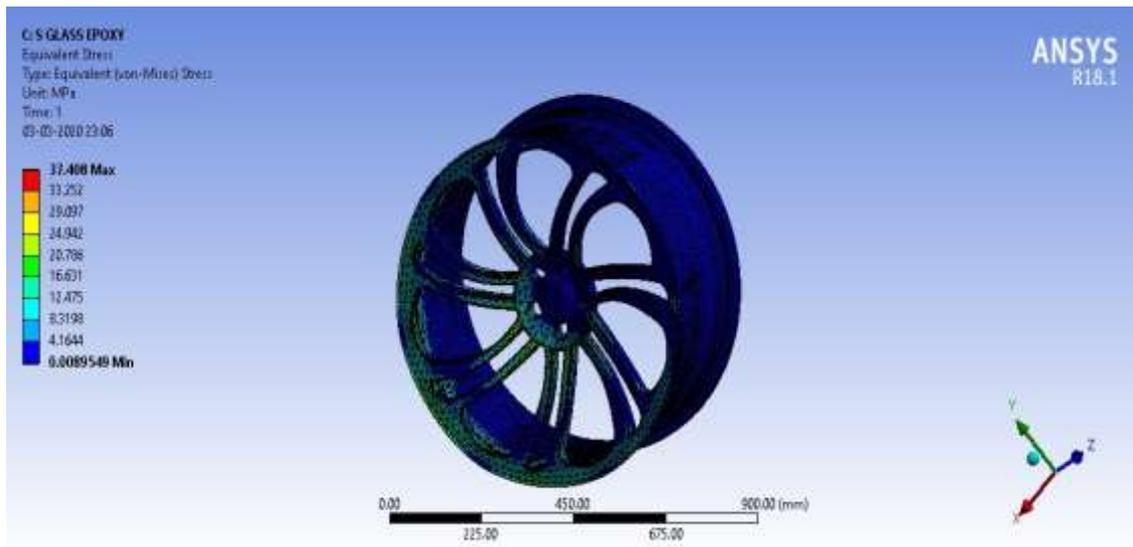
Figure 12 Distribution of equivalent Von-mises stress in wheel rim for S-Glass epoxy material
