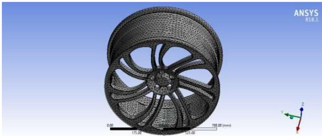
Figure 2 Exclusive finite element model of automobile wheel rim
