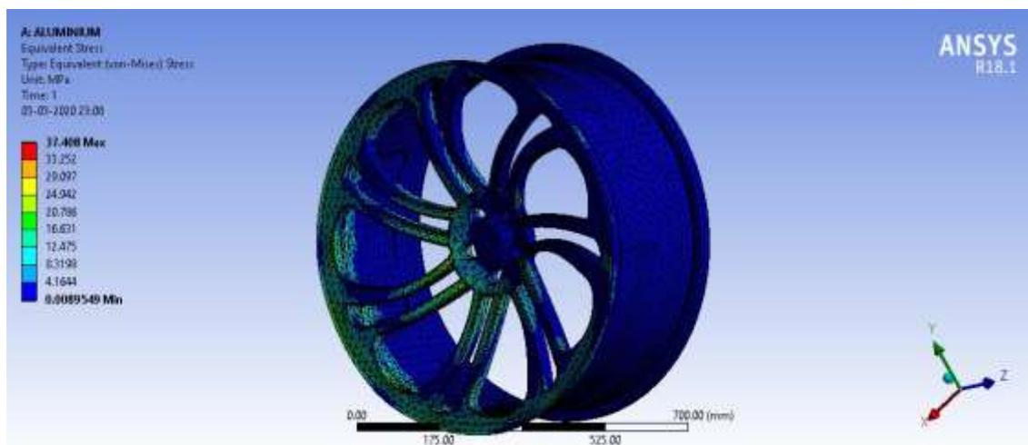
Figure 11 Equivalent Von-mises stress distribution in Aluminium Alloy 6061 wheel rim
