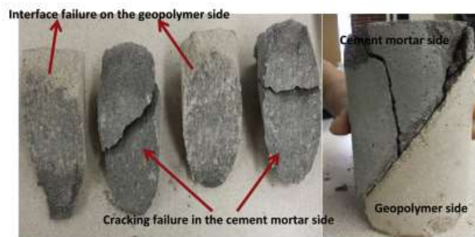
Figure:13 Failure mode of slant shear test with line of interface at 30^\circ between Metakaolin based Geopolymer Mortar and conventional mortar.(13)
