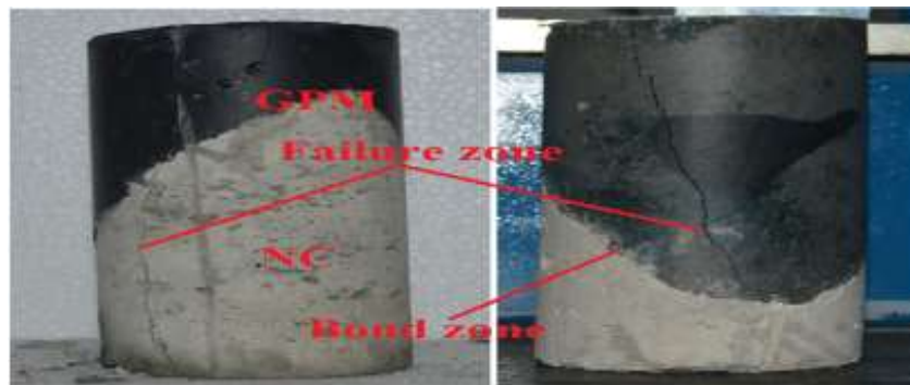
Figure: 20 Typical failure modes of Geopolymer mortar.(15)
