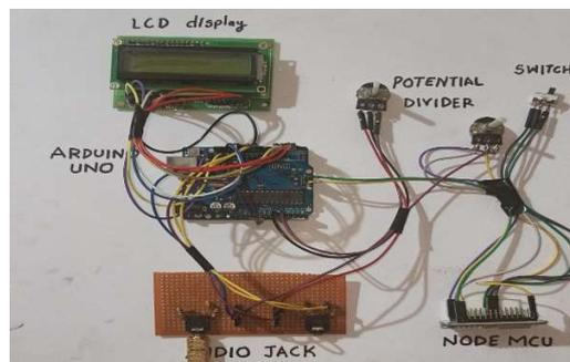
Figure 2. Components used in hardware section
