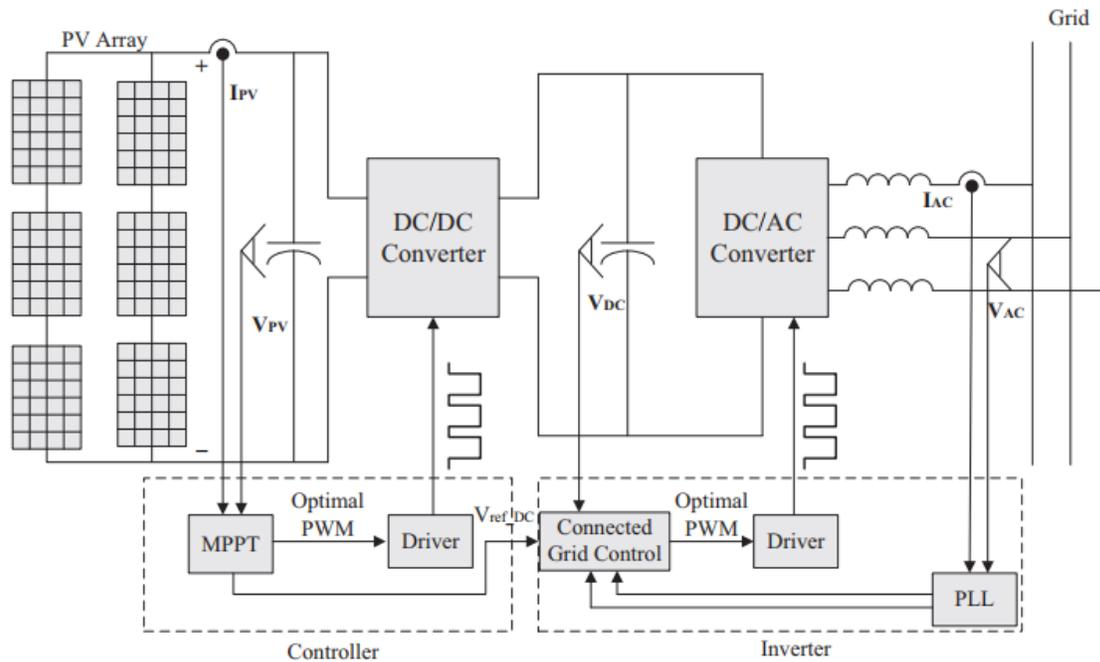
Figure 1: Grid Connected PV array[15]
