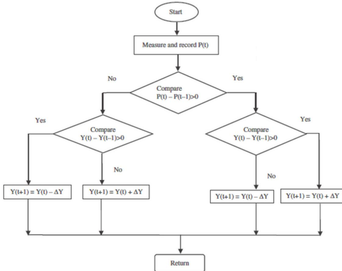
Figure 3: Flowchart of MPPT algorithm
