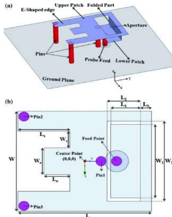
Figure 2. Microstrip radiating patch with shorting pins
