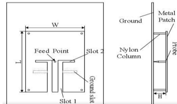
Figure 3. Microstrip patch with slots on the top layer
