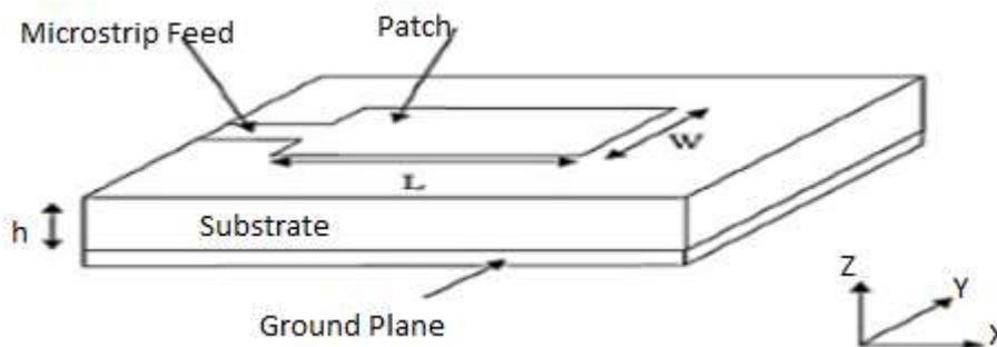
Figure 1. Three Dimensional View of Microstrip Patch Antenna
