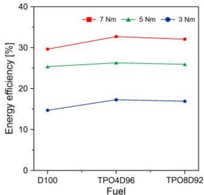
Figure 3. Energy efficiency.
