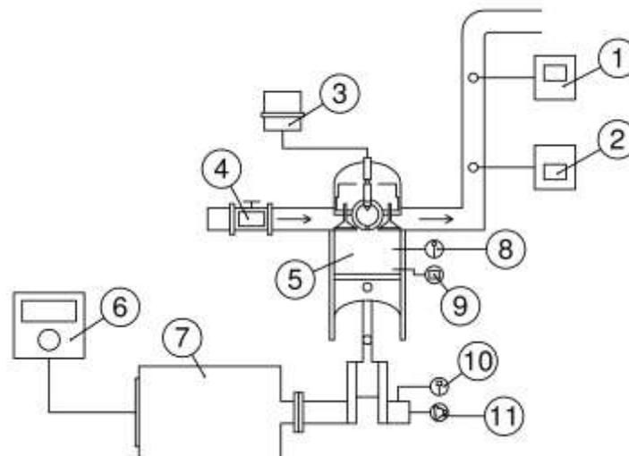
1. PCA® 400, 2. BrainBee AGS-688, 3. Fuel tank, 4. Intake air meter, 5. Engine, 6. Control Panel, 7. Dynamometer, 8. Thermocouple, 9. Cylinder pressure sensor, 10. Encoder, 11. Torque meter.
