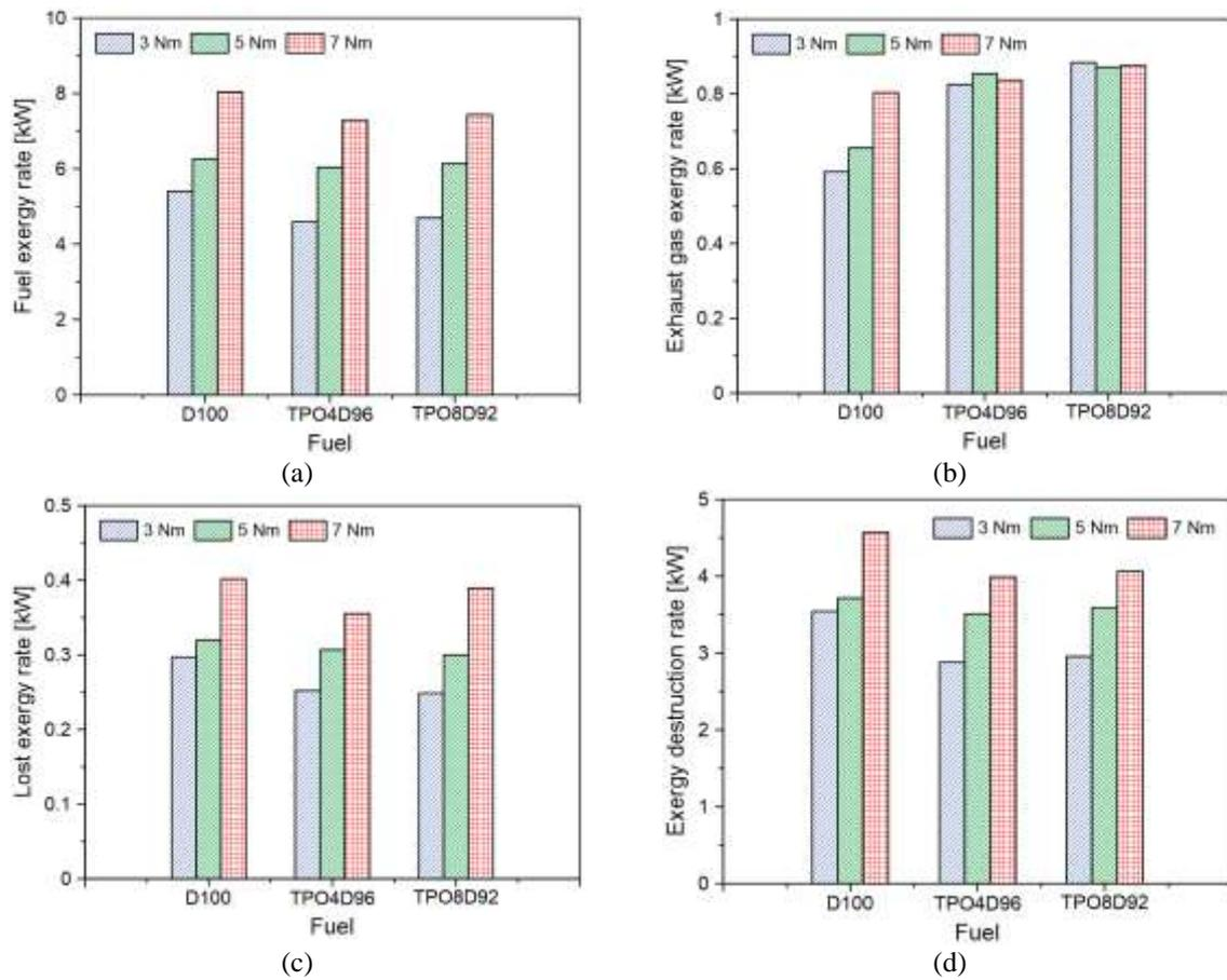
Figure 4. Analysis of exergy flow rates for D100, TPO4D96, and TPO8D92 fuel blends, (a) Fuel exergy rate, (b) Exhaust gas exergy rate, (c) Lost exergy rate and (d) Exergy destruction rate.
