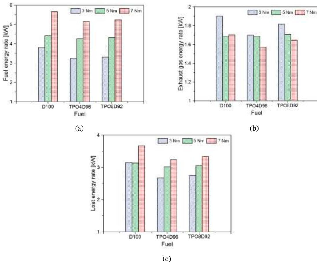
Figure 2. Analysis of energy flow rates for D100, TPO4D96 and TPO8D92 fuel blends, (a) Fuel energy rate, (b) Exhaust gas energy rate, and (c) Lost energy rate.
