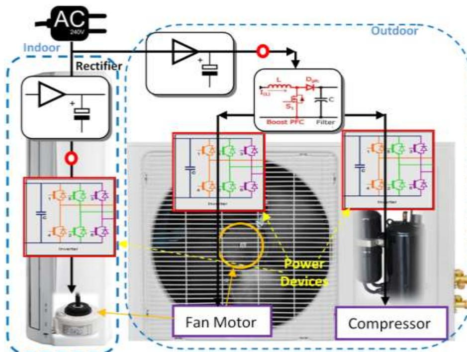
Fig. 6. Block diagram of an air-conditioner of a variable-speed compressor/motor.
