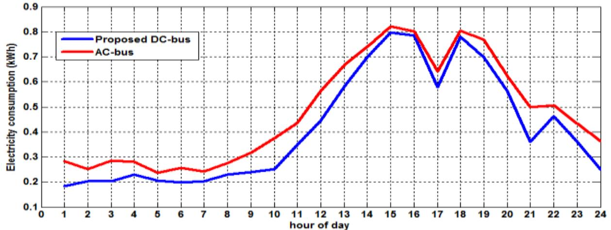
Fig. 8: Air-conditioner energy consumption over a day.
