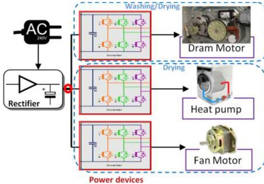
Fig. 9. Block diagram of the speed-controlled motor-driven appliance (Washing Machine).
