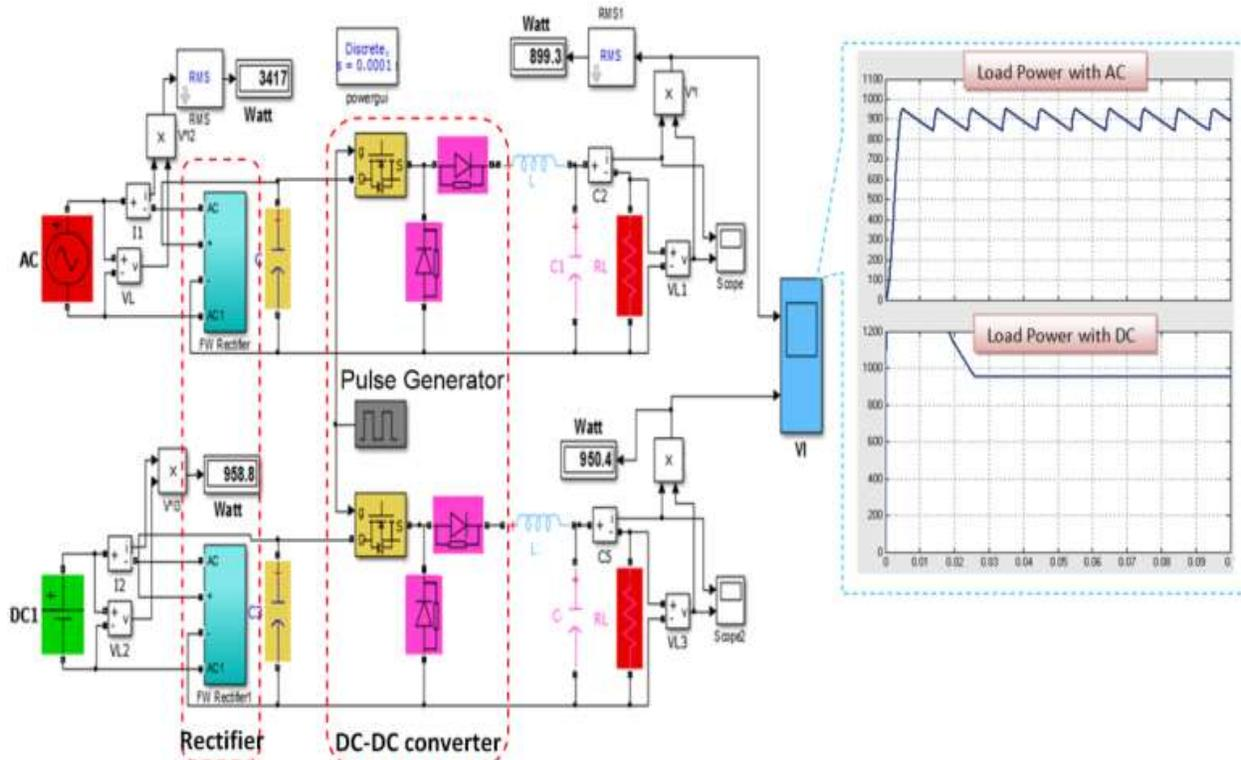
Fig. 2. AC vs. DC as a power source applied at Electronic load, and output waveform
