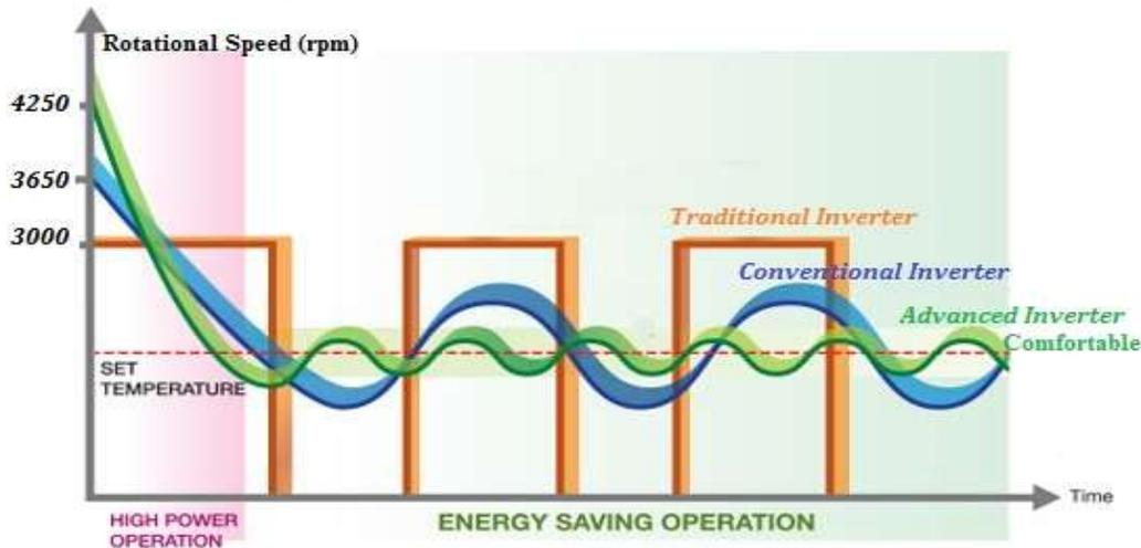
Fig. 5. Variable speed-based compressor operation as compared with a traditional one.
