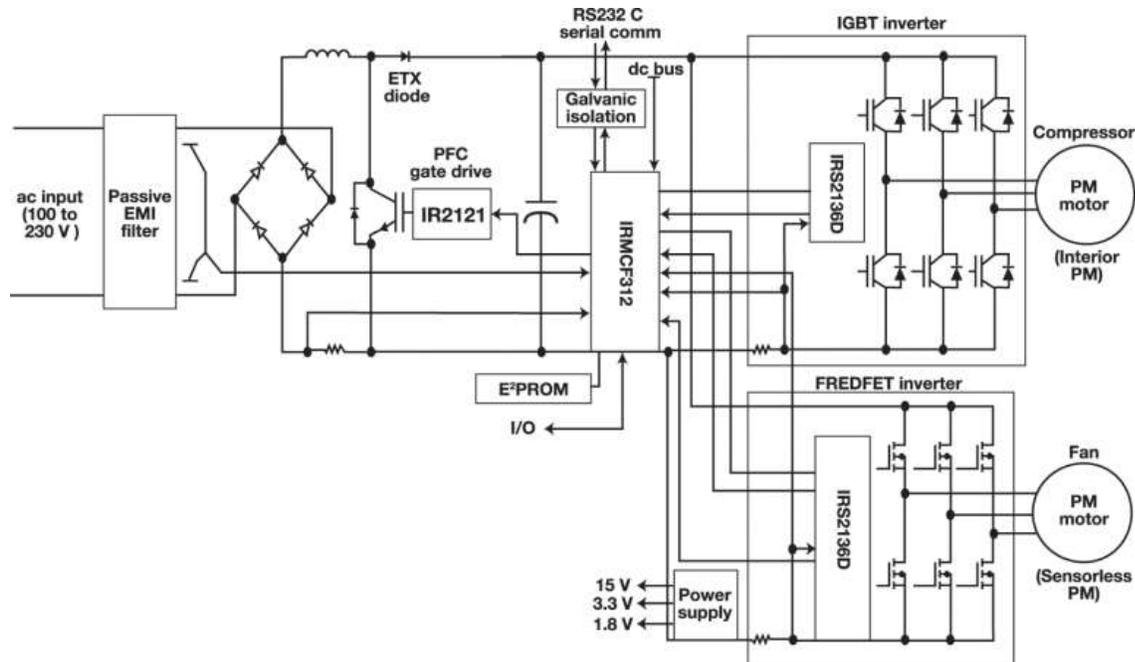
Fig. 7. A generic schematic diagram of an air-conditioner with a variable-speed compressor/motor.
