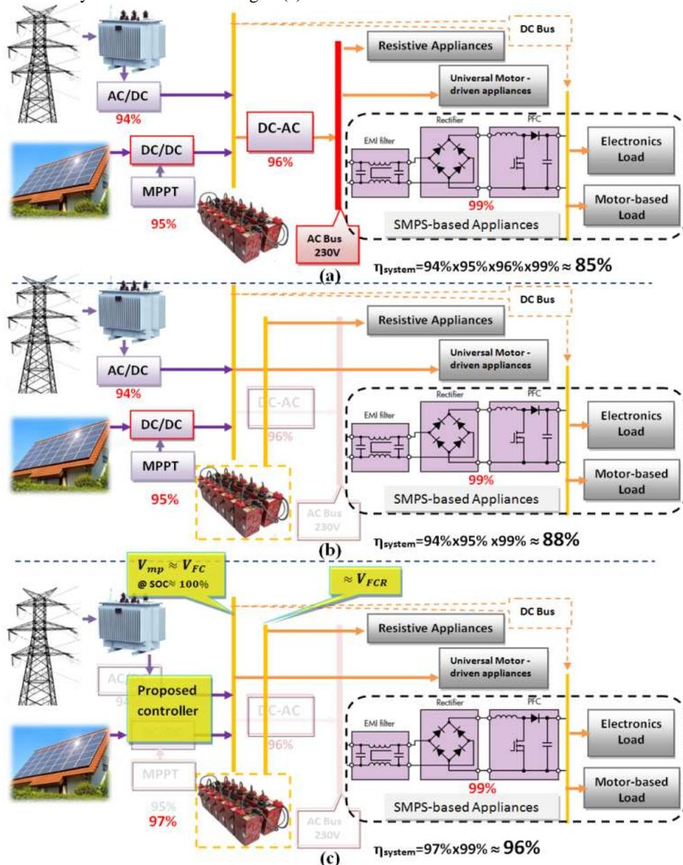
Fig. 1. DC microgrid with Storage topologies: (a) ON-grid traditional with DC distribution includes AC bus, (b) solar farm power source and DC distribution with no inverters, (c) recommended DC distribution system for recent household appliances.
