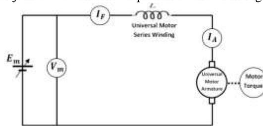
Fig. 3. DC-powered universal motor joined to a constant torque.
