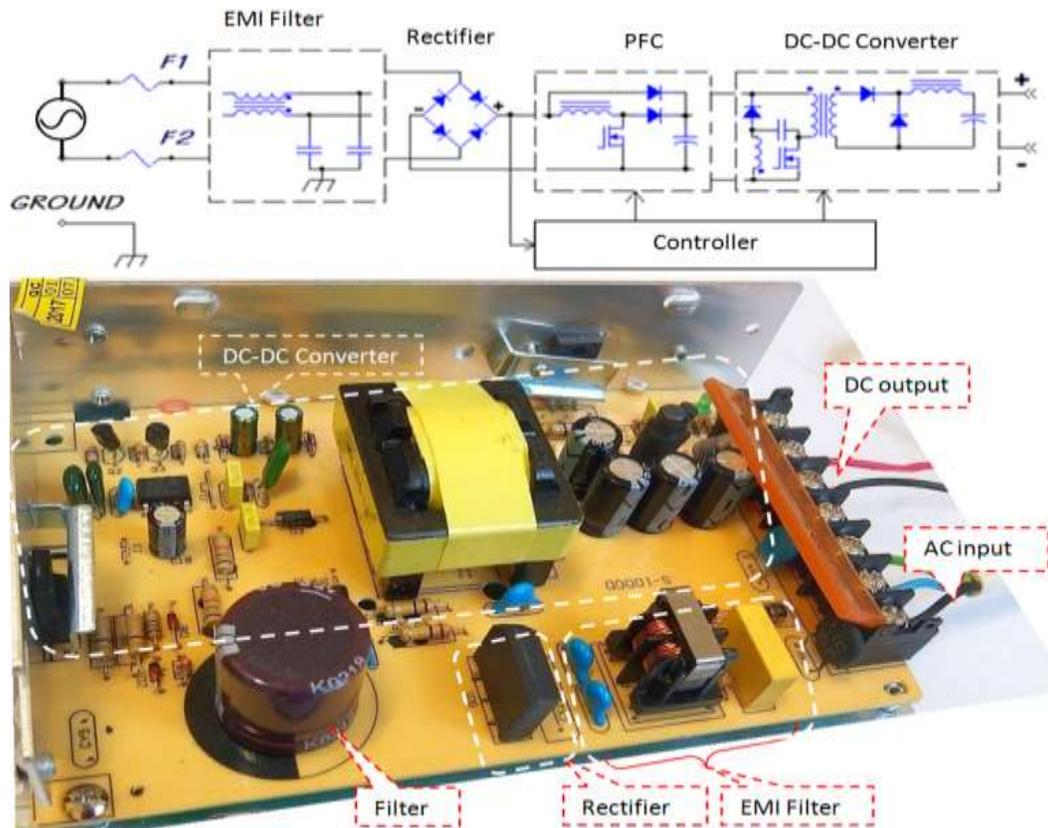
Fig. 4. The conceptual circuit diagram of a typical SMPS.
